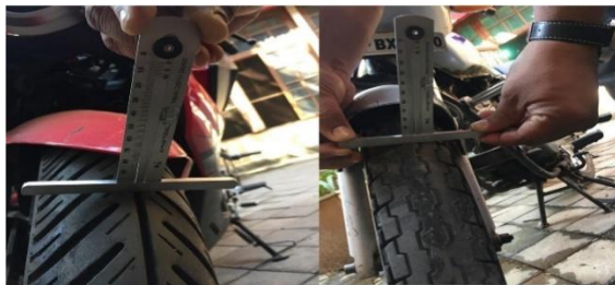
Figure 1: Tyre Ridges Depth Examination with Tyre Tread Depth Gauge
