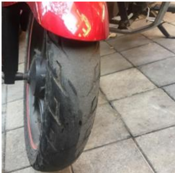
Figure 2: Tyre With No Ridges In Centre
